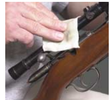
8. Wipe all exterior metal with an oiled rag.
