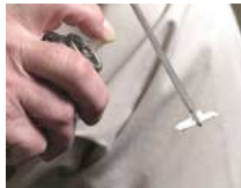
7. When the bore is clean, wipe with a clean patch that is lightly oiled.
