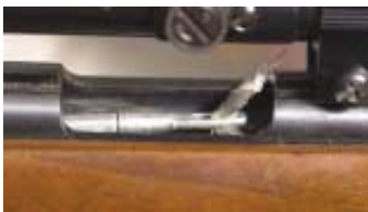
5. Put a clean, dry patch on the rod and wipe the bore.
