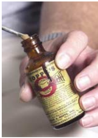
2. Put a cloth patch on the cleaning rod and dampen with a bore-cleaning solvent.
