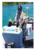
Thousands of geographically referenced depth points are collected to describe the area in as much detail as possible. As the driver navigates the boat along a transect, the datalogger records the coordinates along with a water depth every three seconds.
